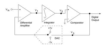
Figure 2. 1<sup>st</sup>-order Delta-Sigma Modulator
